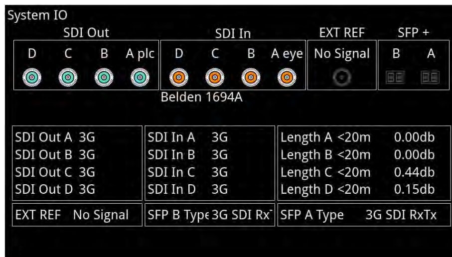
Figure 5-8: System IO Instrument Showing All 3G HD-SDI Out and HD-SDI In BNC Connectors In Use
