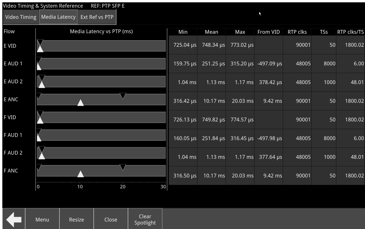
Figure 12-10: Media Latency Tab of the Video Timing & System Reference Instrument (IP 2110 Boot Mode)
