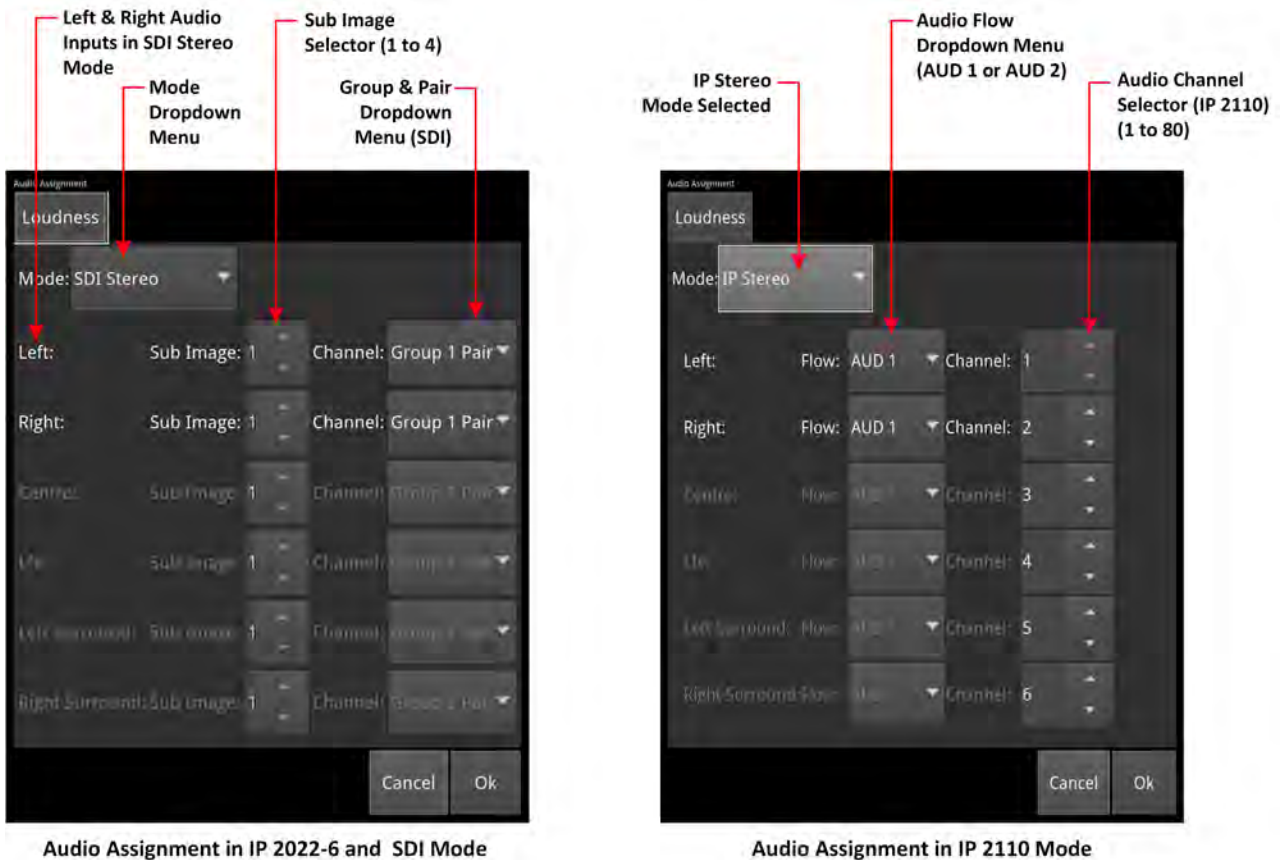
Figure 10-11: Audio Assignment for Loudness Input in IP 2022-6 / SDI (Optional) and IP 2110 Boot Modes
