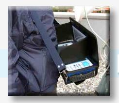
The sun-light-shield flap allows an even better visibility of the high brightness display.
