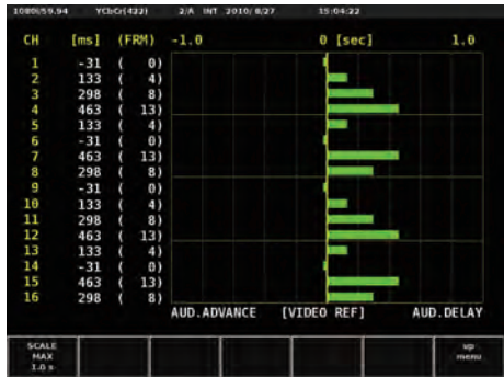
Lip sync display (when the LV 5770SER41 and LT 4400SER01 are installed)
