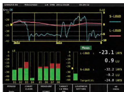
Simultaneous Loudness Measurement on Two Signals
