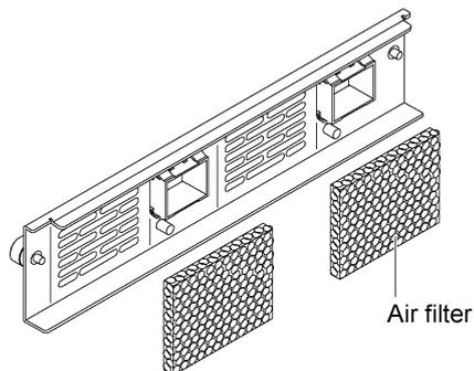
**3. Wash the air filter with mild detergent and water, or remove the dust with a vacuum cleaner.**
