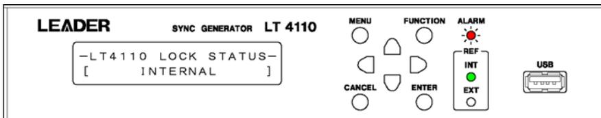
The ALARM LED at the upper right of the front panel blinks in the following situations.
