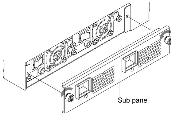
**3. Turn the power supply unit screws counterclockwise, and pull out the unit.**
