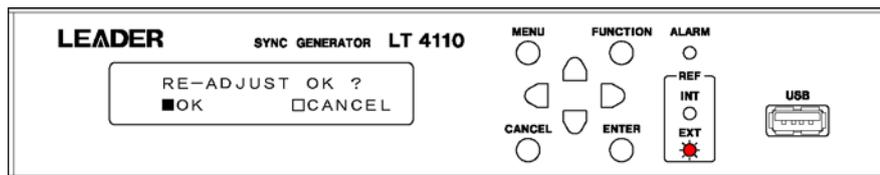
Relocking takes a few seconds, and the output signal becomes discontinuous.
