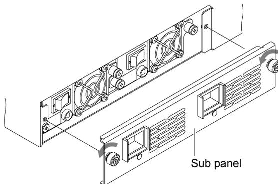
**2. Remove the two air filters from the sub panel.**
