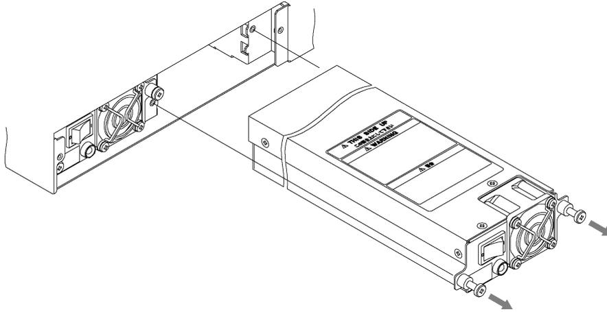
**4. Check that the power switch of the new power supply unit is off (○), and insert the unit.**
