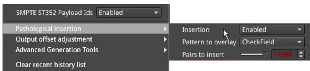
Figure 6-7: Generator - Pathological Signal Insertion Options
