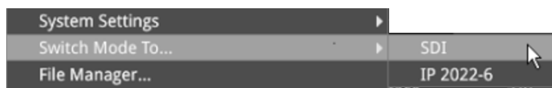
Figure 3-15: Switching Between Qx Boot Modes
