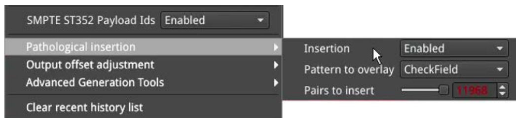
Figure 6-9: Generator - Pathological Signal Insertion Options
