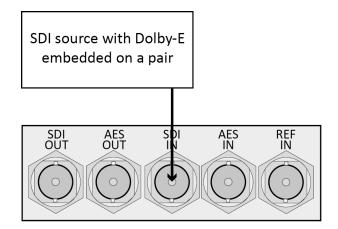
In this example, the SDI signal contains embedded audio with Dolby E present on one or more audio pairs. The Sx instrument needs to lock its internal audio clock to the SDI signal **Generator** - **GenLock** - **GenLock Source** - **Input-1** and the Dolby Timing source should be set to **SDI**.
