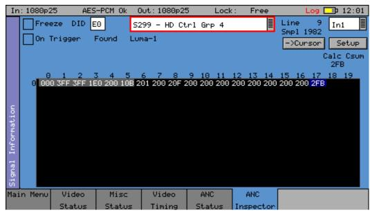
The SDI Data Option **PHSXOSD** allows Ancillary data packets to be detected and checked for errors.
