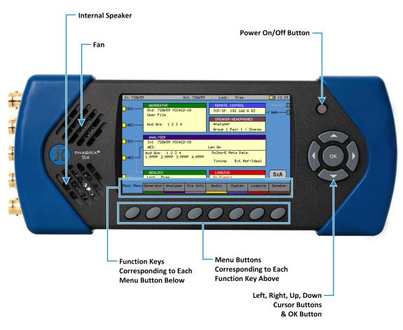
The front panel provides access to the TFT Display and menu system.
