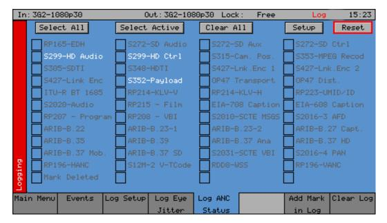
The Log ANC Status menu allows customization of which ANC packets to log for changes in status (e.g., Present, Checksum Error, Missing, Parity Error). Individual checkboxes are provided to determine which packet DID/SDID combinations are logged.
