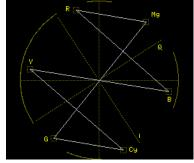
The Vectorscope allows you to check the hue, saturation and phase of the selected input. Controls are provided to allow you to select the line (s) to be monitored (ideal for checking any embedded test pattern in the selected feed), the field to be checked and the graticule scale.
