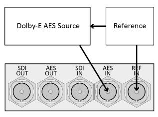
In the example above, the AES signal contains a Dolby E stream. The Sx instrument needs to lock its internal audio clock to the external reference signal **Generator**  $\rightarrow$  **GenLock**  $\rightarrow$  **GenLock Source**  $\rightarrow$  **1Ref** and the Dolby Timing source should be set to **Ext.Ref**. The AES source *must* be locked to the same reference as the Sx.
