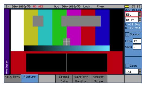
AV Delay measurement (**PHSXO-AVD**) is available in the Picture instrument. Measurement of two AV Delay test patterns is supported:
