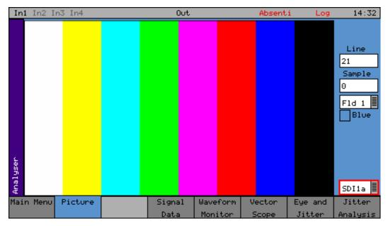
With **Picture** selected, the video picture is displayed in a window as a down-converted display. The picture will automatically view the horizontal or vertical blanking areas if the line or sample values are in the blanking area.
