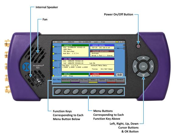
The front panel provides access to the TFT Display and menu system.
