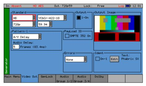
The AV Delay Generator produces an adapted EBU Tech 3305 AV Sync *clapperboard* Test Pattern. This is compatible with third party AV delay analyzers such as the LAWO V\_pro8.
