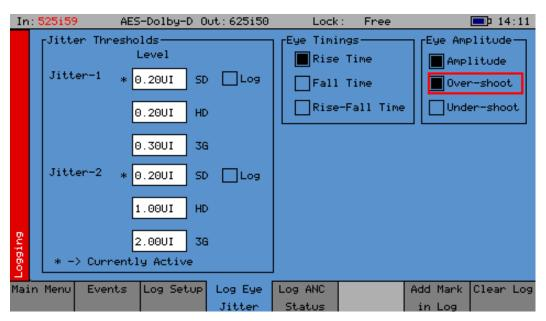
The **Log Eye Jitter** menu allows Eye Jitter events to be logged.
