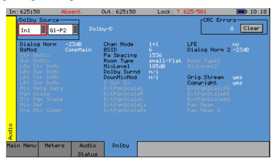
When Dolby Digital metadata is analyzed this displays channel configuration and limited metadata that is sent with Dolby Digital.
