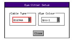
The **Setup** button opens a dialog box allowing the eye color and cable type to be specified.
