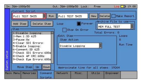
The Command Script and Reports option (**PHSXOS**) allows a series of predefined actions to be run through within the PHABRIX Sx using a script stored in internal memory.
