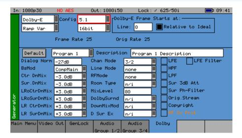
The Dolby generation capability provides broadcast engineers with a highly functional set of tools for Dolby E, Dolby Digital and Dolby Digital Plus streaming. It is unique in being the world's first metadata Dolby generator with editable profiles.
