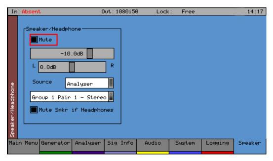
The **Speaker** menu controls which audio pair can be heard on the loudspeakers and headphone output of the Sx instrument. The Sx instrument contains a stereo loudspeaker and associated stereo headphone socket which can be connected to any of the audio input or output channels or pairs.
