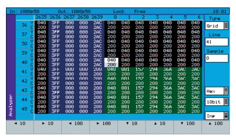
The SDI Data Display and VANC/ANC Inspector option (**PHSXOSD**) provides the engineer with a detailed view of the data words contained within the SDI stream. This allows the analysis of complex
