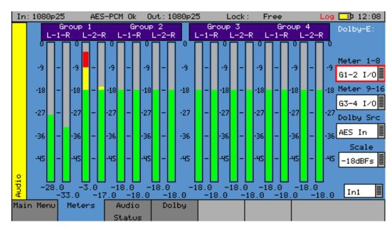
The audio **Meters** menu displays up to 16 audio channels. The source for each block of eight meters may be independently set to allow simultaneous metering of eight inputs and eightoutputs or all 16 channels in an embedded SDI stream.
