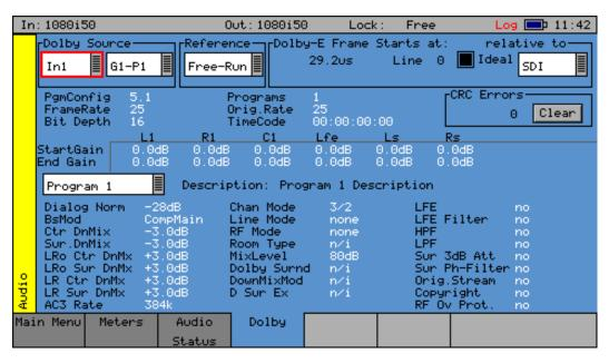
This displays the Program configuration (5.1+2 etc.), the number of programs in the metadata, the frame rates and bit depths and timecode if present.
