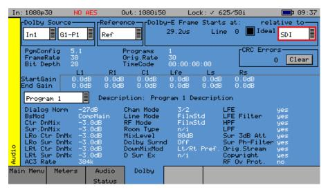
The Dolby audio may be monitored from any of the SDI input embedded audio channel pairs or the AES input. Peak audio levels are also displayed for Dolby E.
