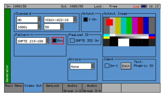
The Sx instrument can create video test signals for all supported SD-SDI, HD-SDI, 3G-SDI and 2K-SDI output standards including the 3 GHz standards at 1080p / 50 / 59 / 60. It will support Y,Cr,Cb, RGB and XYZ formats as well as RGB formats.
