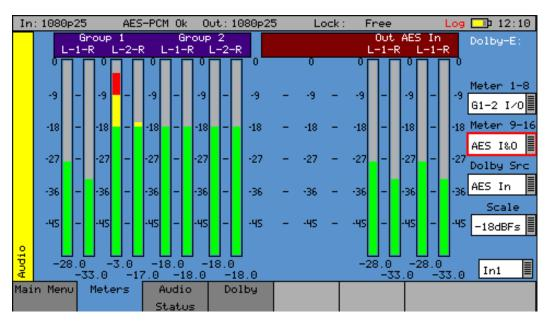
If AES inputs or outputs are present, then these may also be metered. At the bottom of each meter is the current audio level for that channel in dBFS (decibels relative to 0 dB full-scale).
