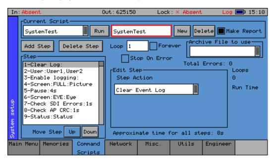
The **Command Scripts** menu allows the Sx instrument to run predefined scripts. This can be used to automate testing of signals.
