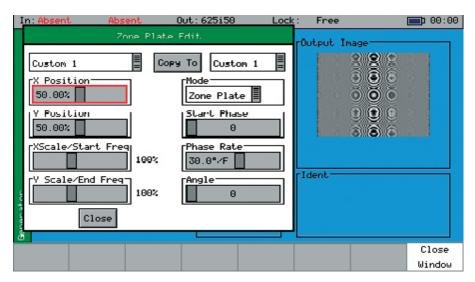
The Zone Plate Generator option (**PHSXOZ**) adds a range of preprogrammed zone plate patterns along with user-defined controls over several parameters which can be saved to custom buffers.
