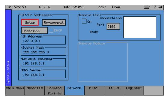
PHABRIX Sx is fully network compatible and has a complete network interface to allow control of any Sx instrument from any other unit.
