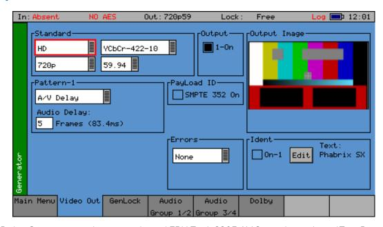
The AV Delay Generator produces an adapted EBU Tech 3305 AV Sync *clapperboard* Test Pattern. An audio delay offset with respect to video of up to +/- 40 frames can be applied in increments of one frame.
