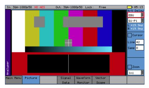
AV Delay measurement (**PHSXO-AVD**) is available in the Picture instrument. Measurement of two AV Delay test patterns is supported:
