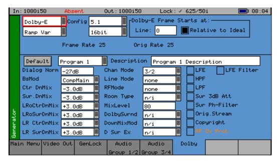
The Sx instrument Dolby Generator software option (**PHSXO-DAG**) allows the generation of Dolby E, Dolby Digital and Dolby Digital Plus pre-encoded test signals to check that they are transferred transparently through the broadcast chain unaffected by routers/switchers, satellite links, etc.
