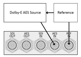
In the example above, the AES signal contains a Dolby E stream. The Sx instrument needs to lock its internal audio clock to the external reference signal **Generator**  $\rightarrow$  **GenLock**  $\rightarrow$  **GenLock Source**  $\rightarrow$  **1Ref** and the Dolby Timing source should be set to **Ext.Ref**. The AES source *must* be locked to the same reference as the Sx.
