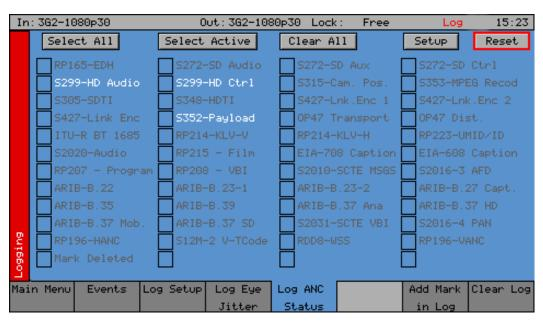
The Log ANC Status menu allows customization of which ANC packets to log for changes in status (e.g., Present, Checksum Error, Missing, Parity Error). Individual checkboxes are provided to determine which packet DID/SDID combinations are logged.
