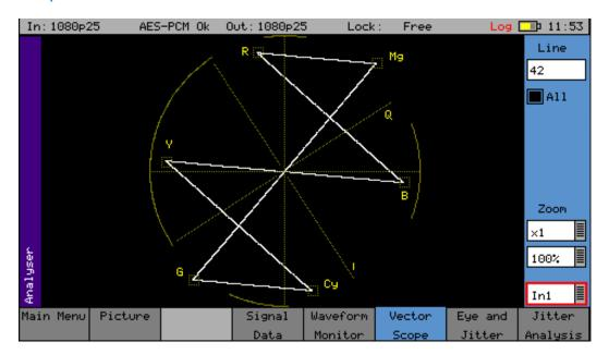
The Vectorscope menu displays the selected input in the form of a vectorscope. This may be set to show either the 100% bar positions or 75% positions. The color bar position boxes will change according to the color space for the current input video standard.
