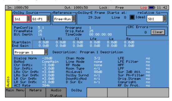
The **Dolby** Analysis option allows display of the Dolby E metadata present in the selected audio stream and determines whether the Dolby E packet is timed correctly on the SDI video stream.
