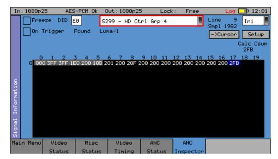
The SDI Data Option **PHSXOSD** allows Ancillary data packets to be detected and checked for errors. The ANC Inspector menu displays details of the ANC packets.
