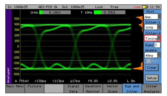
The **Eye and Jitter** menu displays the selected input in the form of an *Eye Pattern* display.
