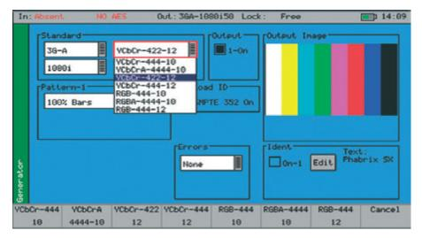
This option (**PHSXOF**) provides advanced formats including: 4:2:2 YUV, 4:4:4 RGB and 4:4:4 YUV at 10/12 bit, and 2K formats including: 4:2:2 YCbCr, 4:4:4 RGB' and 4:4:4 YCbCr at 10/12 bit as well as 4:4:4 XYZ at 12-bit. For broadcast manufacturers this option allows rigorous testing of many more formats beyond the standard signals used in traditional broadcasting.
