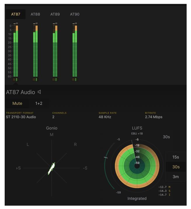
The audio view shows the audioflows belonging to the specific service. The audioflows are displayed in three different sections of the view, through RMS meters, Goniometer and a LUFS radar.
