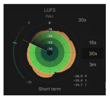
In the bottom right corner there are three time scales, M (Momentary), S (Short-term) and in I (Integrated). The time scales all have different time windows. M - 400ms, S - 3sec, I - from start to present. All three timescales show the present average loudness.
