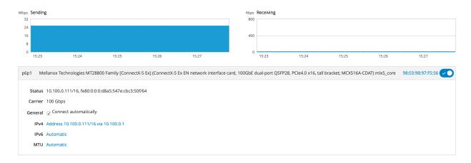
To enable or disable the interface click the switch button in the top right corner. By default all settings are set to automatic, however there is also a possibility to manually configure the IP related settings in this view.
