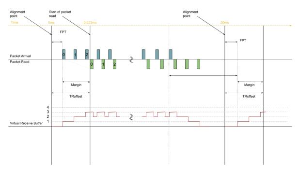
The figure above illustrates the timing model, which puts constraints on the timing of packets on the output of the sending device. The network compatibility model (C), Virtual receiver buffer (VRX) and packet read schedule (PRS) all ensure that the delivery timing is overheld by shaping the transmission.
