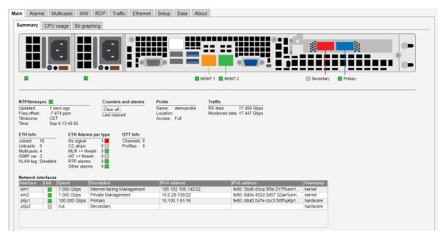
The intention of this page, together with the **alarm list**, is to provide enough information for the operator to immediately see if there is anything seriously wrong with one or more input streams.
