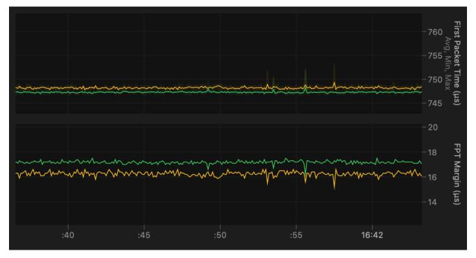
The second two graphs show *First Packet Time* and *FPT Margin*. The *First Packet Time* graph shows the time difference between the packet's timestamp at arrival and the Alignment Point. While the FPT Margin graph shows the time difference between the packet's timestamp at arrival and start of packet read.
