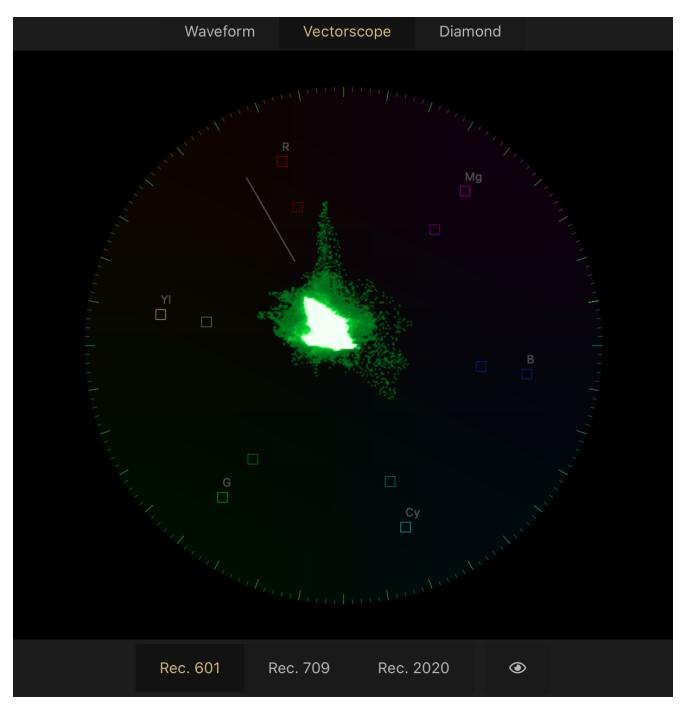
To change the colourimetry, use the buttons at the bottom. Changing the colour space in this view, will change the video picture for all clients. To increase the contrast of the vectorscope, press and hold the eye icon.
