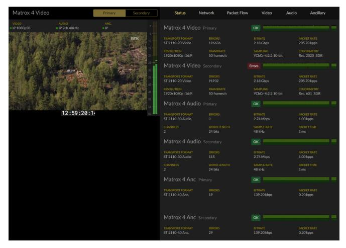
If you have configured and joined more than one class of flows for a service, you have the option to view both classes, in this view named "Primary" and "Secondary". Note that the class names are configurable and can be named as preferred. For more information, see section *"Naming and configuration of flows"*.
