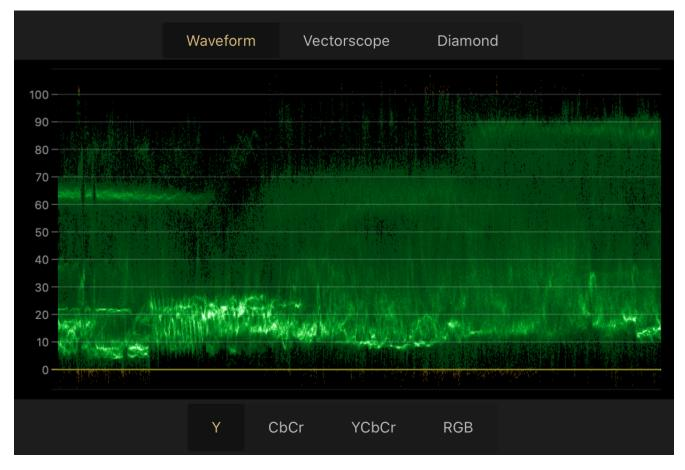
In the waveform scope there are four different displays. Y Displays luminance, CbCr displays color difference, YCbCr combines the first two and RGB shows the red, green, and blue components in the video. The buttons at the bottom of the view makes it easy to select the prefered data.
