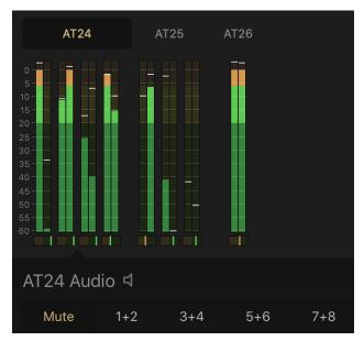
In the screenshot above shows three audio flows, to select one, click on the flow name. The first flow (AT24) contains eight audio channels. The audio channel is set to mute by default, to enable audio, click on the preferred channel pair. Underneath each of the paired RMS meters there is a Microphase meter.
